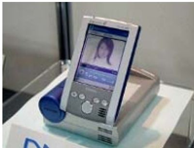
Fuel cells for wireless, mobile computing devices: Toshiba's DMFC-powered PDA on display (left).
